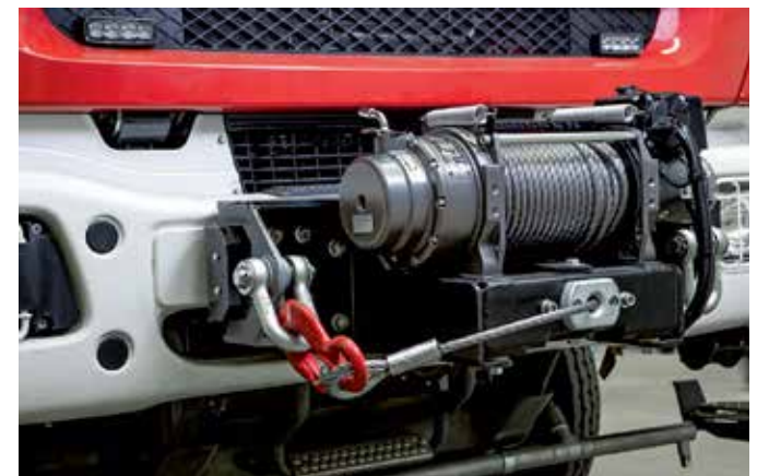
/ Front-mounted winch for technical assistance and self-removal
