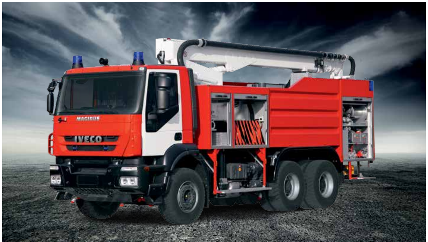
/ Telescopic extinguishing booms enhance the vehicle's tactical abilities for fire-fighting e.g. in industrial plants.
