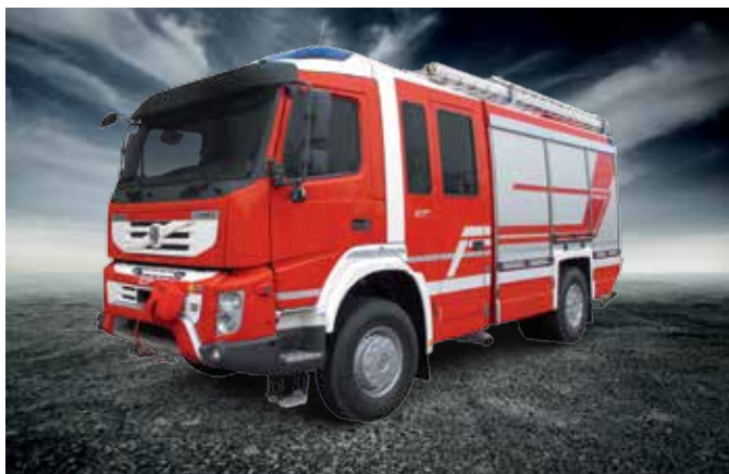
/ Customized Tank pumper with crew compartment 1+8
