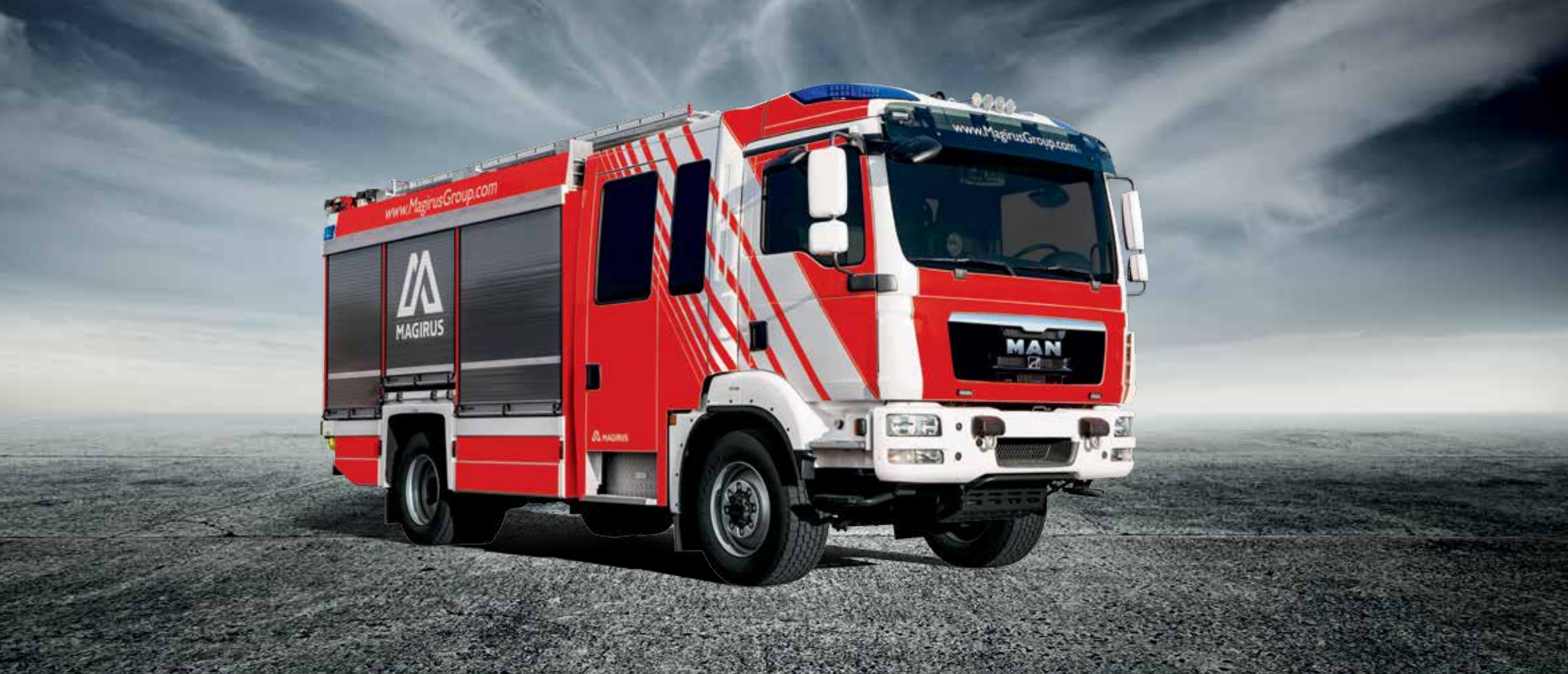
/ 2000 litre class fire-fighting vehicle on MAN 4x4, with Magirus crew compartment in aluminium technology
