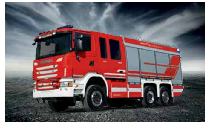
/ GTLF on Scania 4x4, with Magirus crew compartment in aluminium technology
