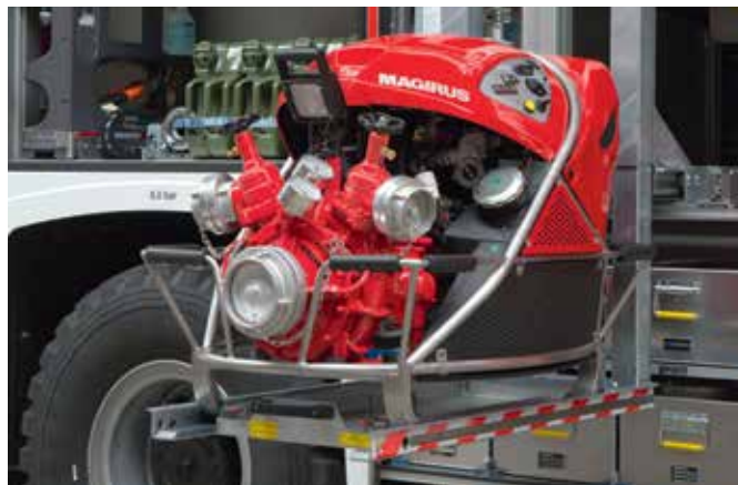
Lowerable fire pump storage for ergonomic removal
