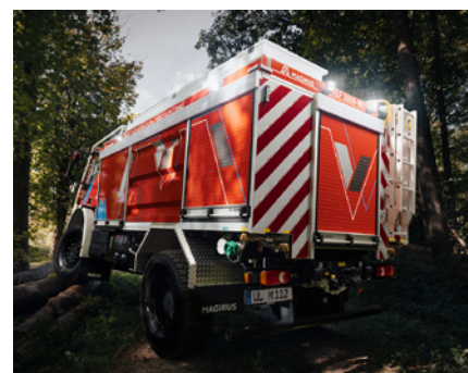
Ideal water tank position for a low center of gravity and balanced weight distribution
