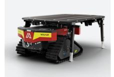
Expandable swap body system incl. airline rails ensures maximum flexibility and safe transport
